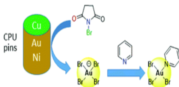
Fig. 3 The growing environmental Risks of E-Waste Fig. 4 Leaching of gold from e-waste Cyanide Boost
